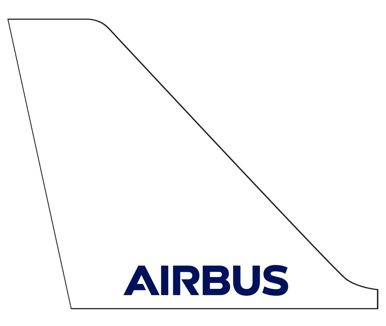
A vertical stabilizer, pictured here, is a crucial part of an aircraft because it provides sufficient directional equilibrium, stability and control. The vertical stabilizer is located on the tail of a plane, and controls "yaw," which is the side-to-side movement of the nose of an aircraft.
